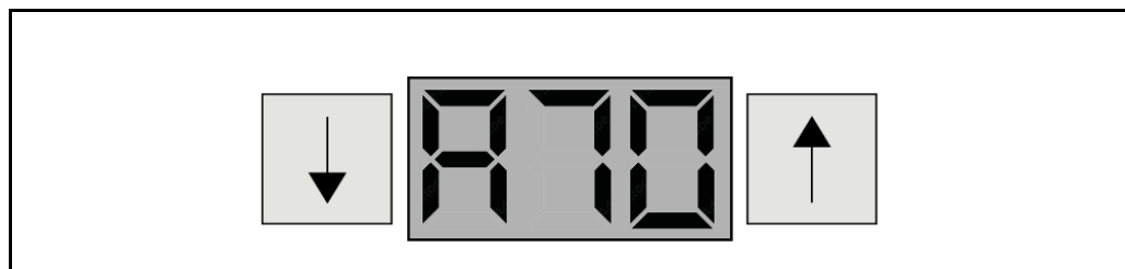
Figure 04: Indication of the battery charging status (70% in the example)
