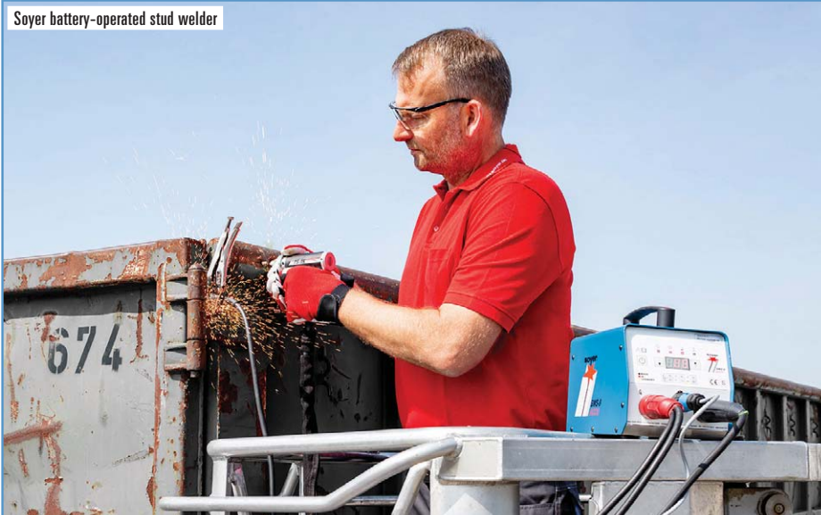
Soyer battery-operated stud welder
