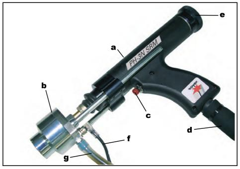
Figure 7: PH-3N SRM stud welding gun
