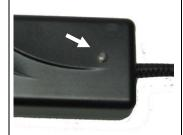
The current state is indicated by a light-emitting diode located on the external battery charger.
