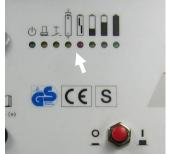
The LED "Supply voltage on" lights up when power is supplied via the external battery charger.
