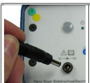
Insert connecting plug of the external battery charger into the connecting socket located at the stud welder's front panel.
