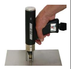
Position welding gun vertically on the workpiece (at a 90-degree angle to the workpiece).
