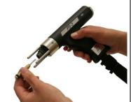
The stud welder must be <u>switched off</u> when installing the stud chuck.
