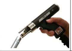
Hand-tighten sleeve nut by means of SW 17 socket wrench.
