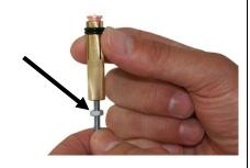
The weld stud must make contact with the stop screw. Adjust stop screw in the stud chuck by turning it until the distance between the top edge of the stud flange and the front edge of the stud chuck equals 1.5 mm.
