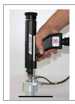
Position welding gun vertically on the workpiece (at a 90degree angle to the workpiece). Check the selected parameters. Start the welding process by pressing the trigger.
